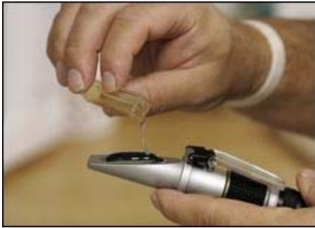
Mark Grigg pours honey onto a refractometer to determine the moisture content of the honey at Silverbow Honey in Moses Lake.
